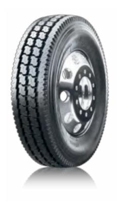
The S768 EFT is a premium closed shoulder drive tire, designed with a wide shoulder featuring tapered lateral edges for enhanced lateral stability. The S768 also features stone ejector buttons that reduce stone retention, and an extra-deep 26/32" tread depth for enhanced tread life.
