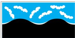
White carbon black sticks better to the body of the tire which creates less friction. This greatly reduces the tire's rolling resistance. White carbon black is more flexible making it better at absorbing shocks from road deformations and improves grip.
