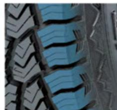
**Aggressive open shoulder tread design:** efficiently expels snow, water, slush, and mud for optimum traction in all-terrain conditions.
